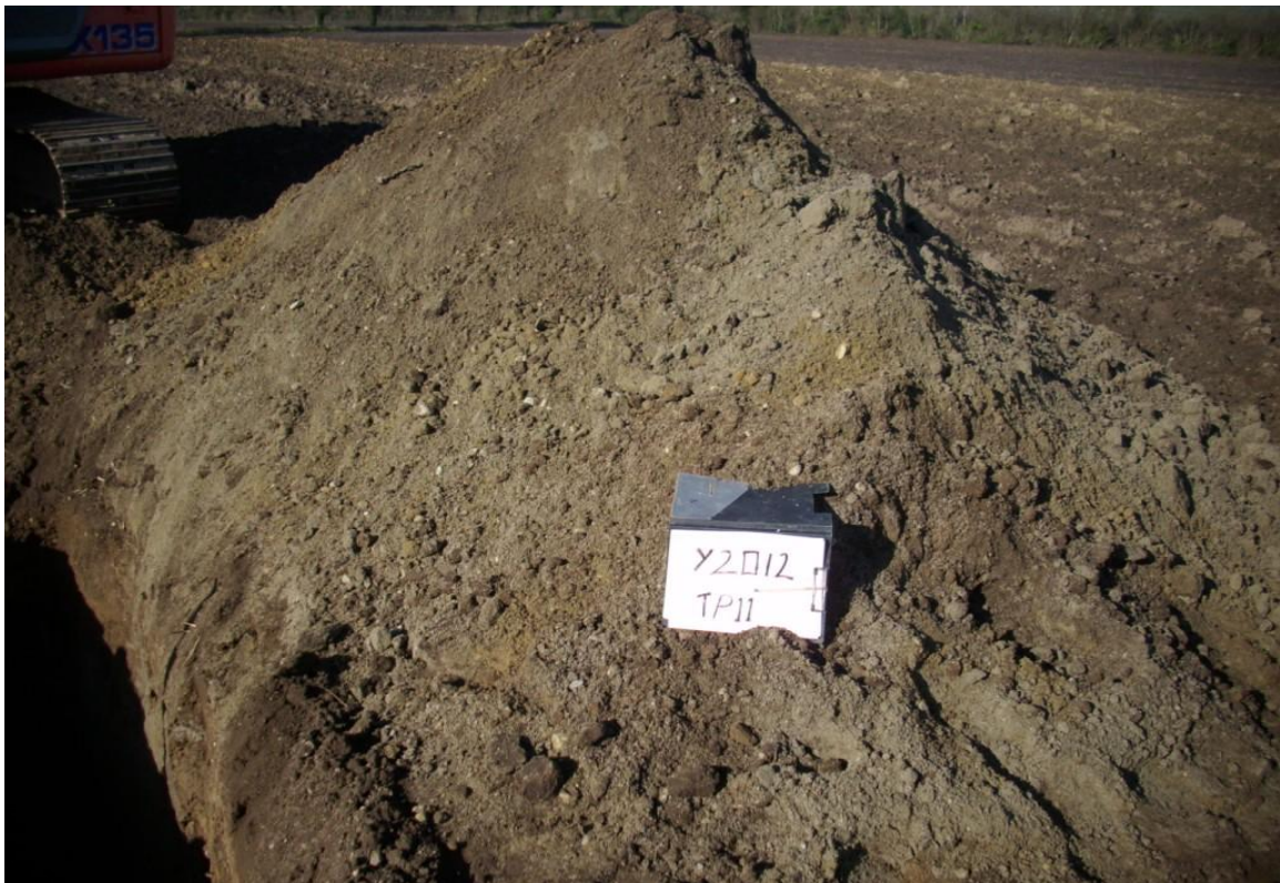
Trial Pit Spoil
