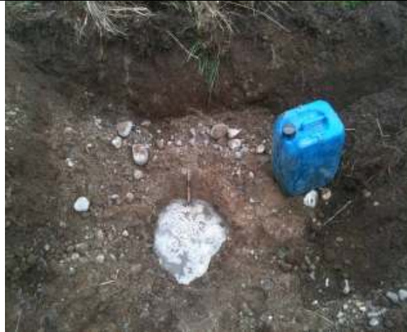
Percolation ("T") Test 2
