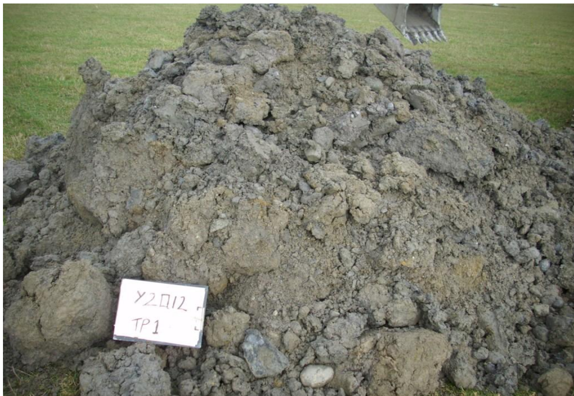
Trial Pit Spoil
