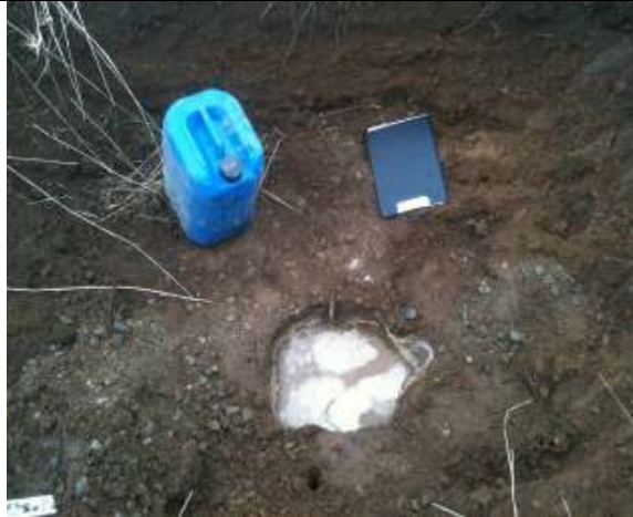
Percolation ("T") Test 1
