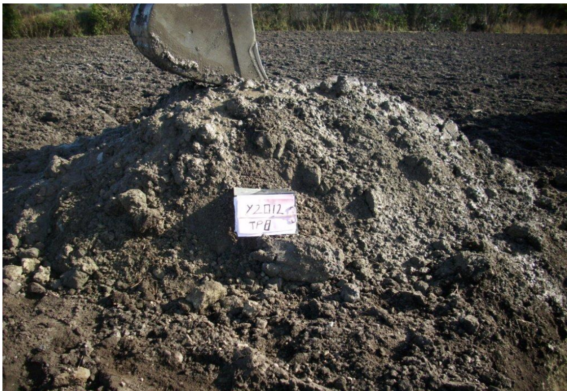
Trial Pit Spoil
