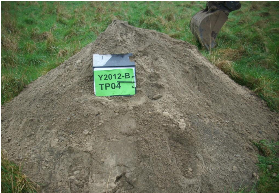
Trial Pit Spoil
