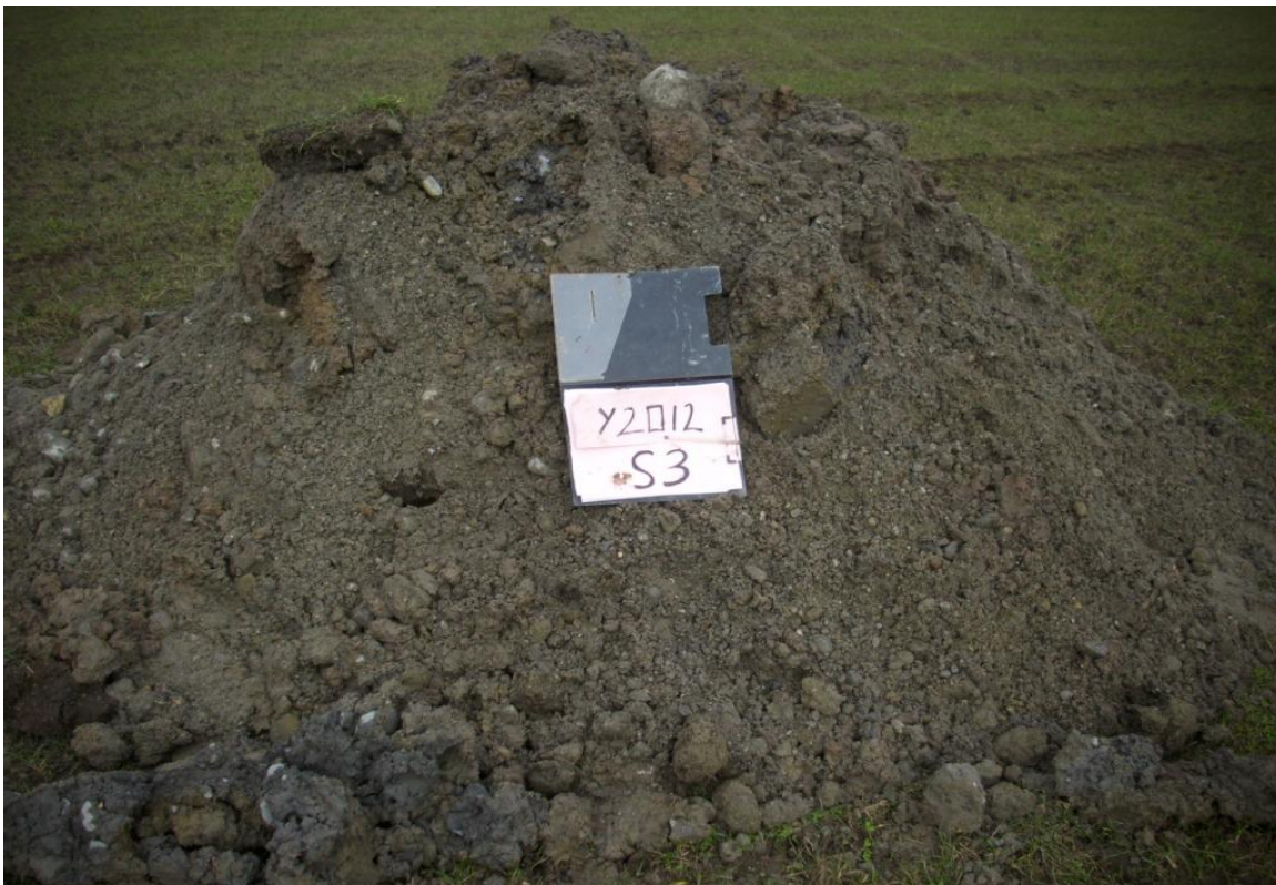
Trial Pit Spoil
