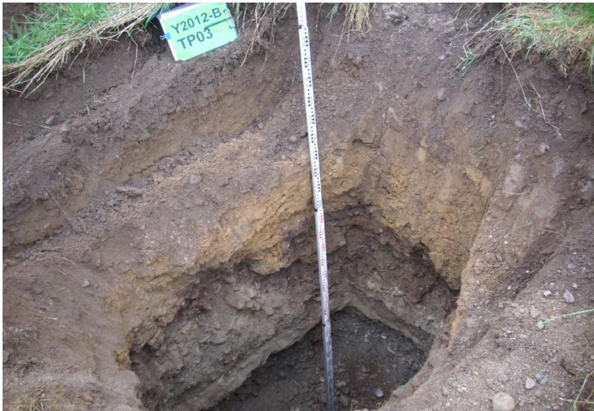
Trial Pit Side/Base
