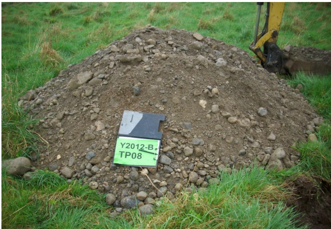
Trial Pit Spoil
