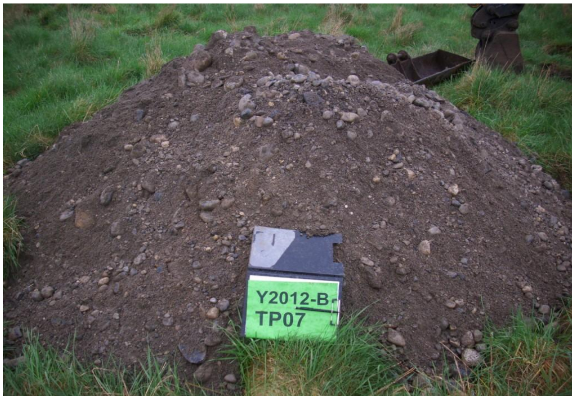
Trial Pit Spoil
