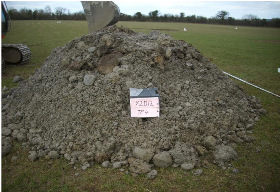
Trial Pit Spoil
