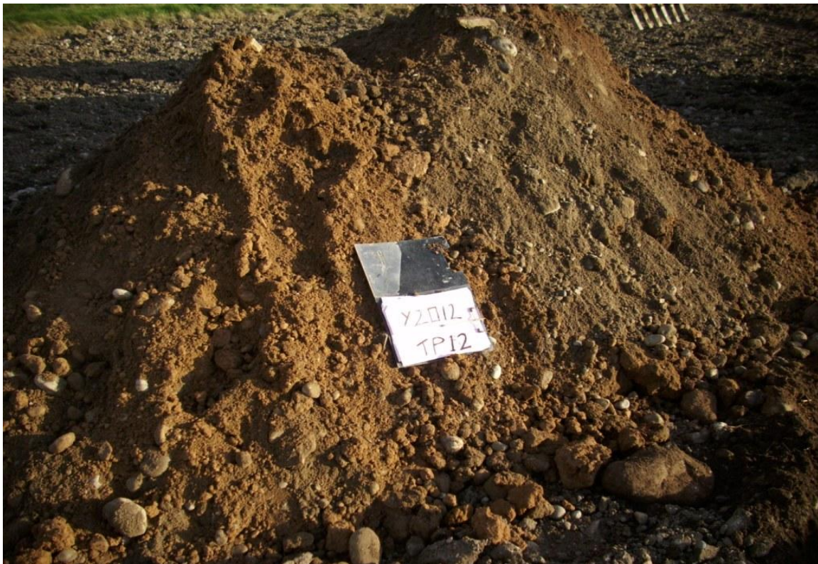
Trial Pit Spoil
