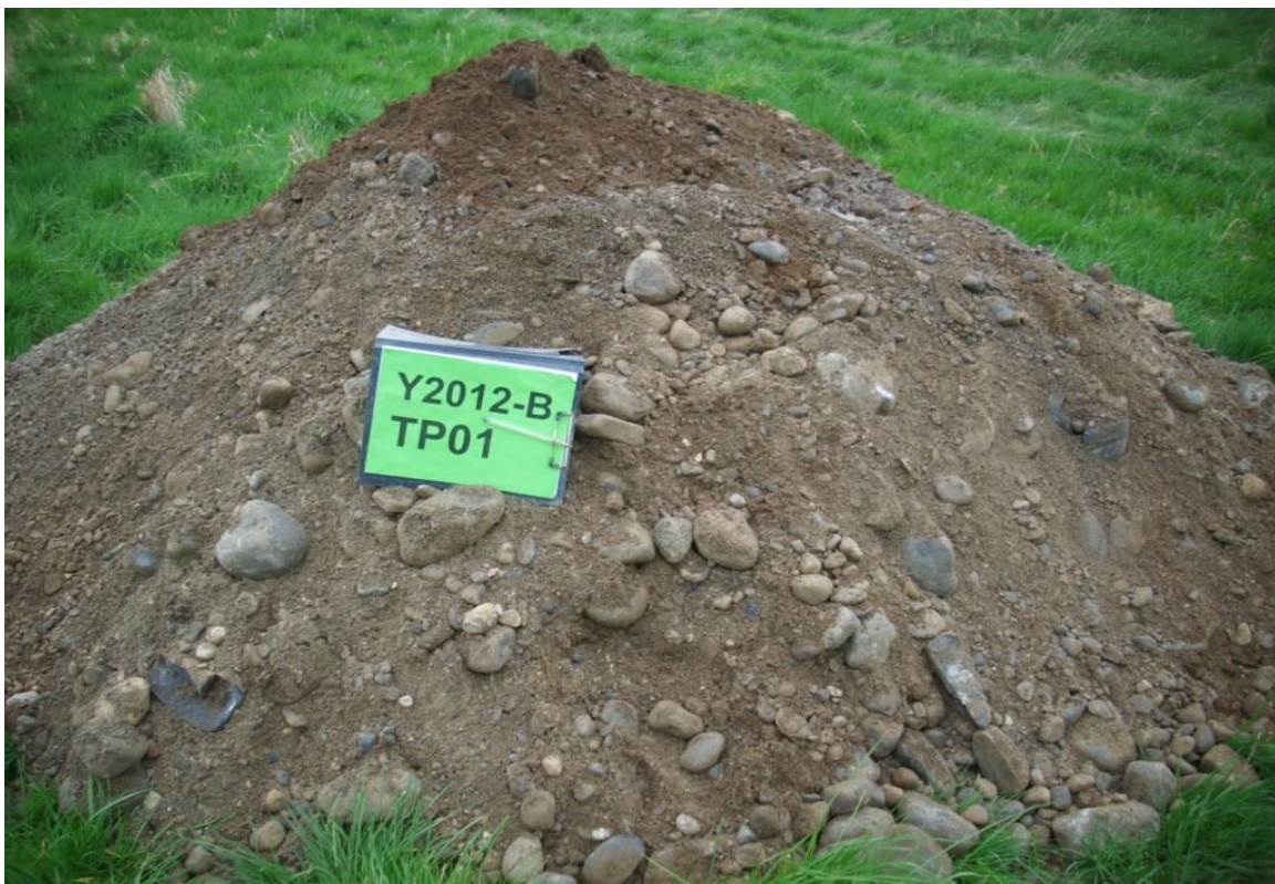
Trial Pit Spoil
